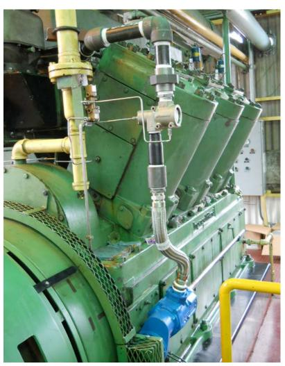
**Low air consumption:** The IR starter required 250 psi and often took over 30 seconds to start; the new T121V requires only 60 psi to achieve maximum starting roll speed and starts engine in less than 10 seconds.
