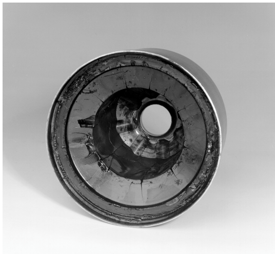
Figure 16 - Centrifuge Rotor Cover from Engine 2 (Third Oil Drain - 1400-2100 Hours)
