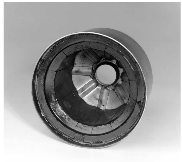
Figure 14. Centrifuge Rotor Cover from Engine 2 (First Oil Drain - 0-700 Hours)
