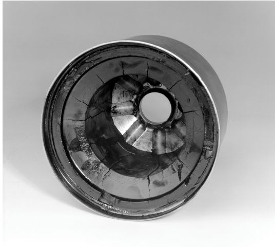
Figure 15 - Centrifuge Rotor Cover from Engine 2 (Second Oil Drain - 700-1400 Hours)
