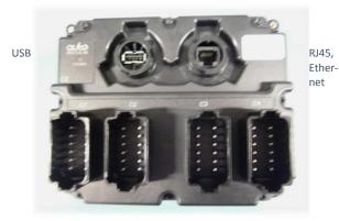
C1: C2: C3: C4: Power Relav1. 109-20 Therm1. CAN, Relay2, Therm2, RIO, AllFaults. RS-485. 101-4 105&21 106-8
