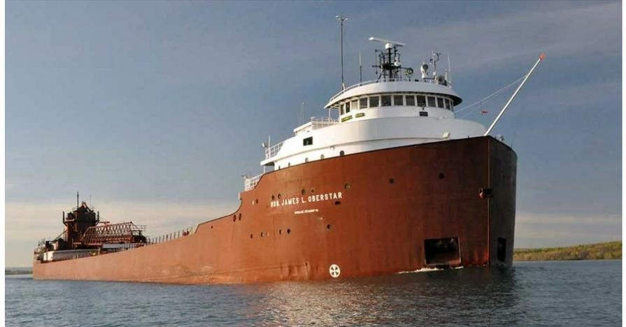
The M/V Honorable James L. Oberstar is an 800' bulk carrier operating on the Great Lakes of Northern America. The vessel is powered by two Bergen B:32:40L diesel engines. The engines clutch in together to a common gearbox to drive a propeller for propulsion and a shaft generator for electrical power.
