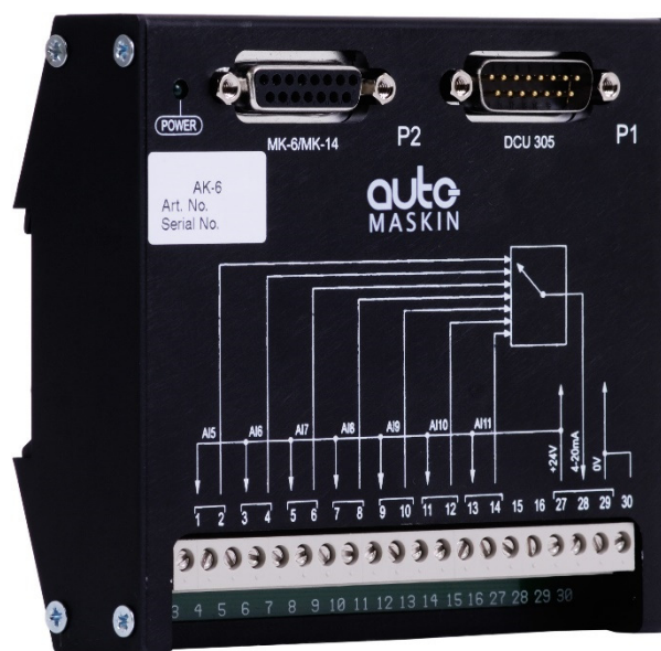
The optional AK-6 analogue card, which adds six 4-20 mA channels to the DCU 305 R3.
