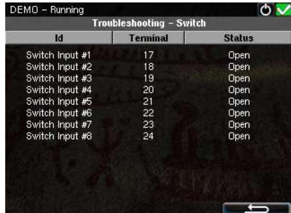
If for instance the troubleshooting screen indicates open, and there is a 24V signal connected to the input channel, then that input channel is broken.
