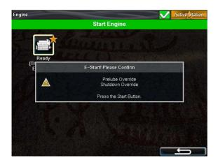
**Note!** Activating E-Start will override any configured Prelube and also set Shutdown Override. The engine will start immediately, and run in a Shutdown Override setting.
