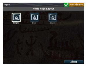
The Home page can use the entire screen for a single engine, or it can be divided into two or four rectangles.
