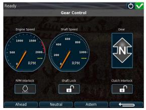
This form is used to inspect transmission related parameters and to request gear changes.
