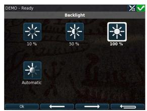
Note that if 10% is selected, the DCU will still switch to 50% backlight intensity while in the menu.
