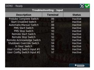
If for instance DCU terminal 89 is measured to 24V, but the troubleshooting screen for that channel indicates 'Inactive', then that input channel is faulty.
