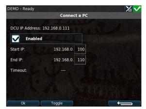
Make sure the DCU IP-address is outside the DHCP Start- and End IPaddress range, by setting the start IP higher or the end IP lower than the DCU IP-address.
