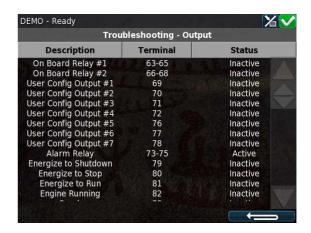
If for instance terminal 81 indicates 'Active' (24V) but a voltmeter indicates that there is no 24V on terminal 81, then that output channel is faulty.
