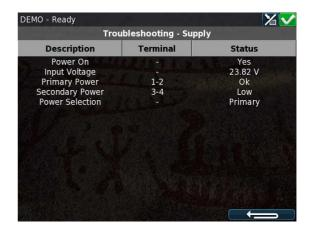
The DCU automatically select its power from either the primary or the secondary supply.
