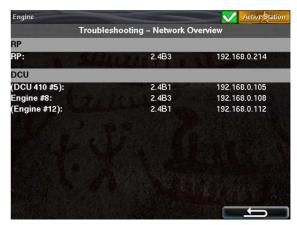
Panels listed in parenthesis are detected on the network but not configured connected to this RP.
