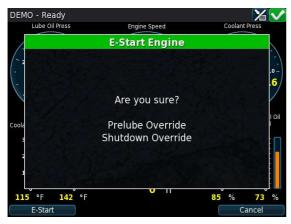
**Note!** Activating E-Start will override any configured Prelube and also set Shutdown Override. The engine will start immediately, and run in a Shutdown Override mode setting.
