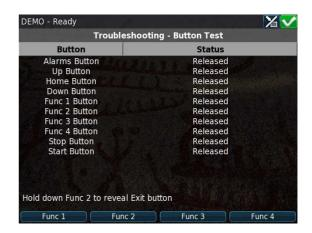
To leave the test, press and hold button Func 2, then press button Func 4.
