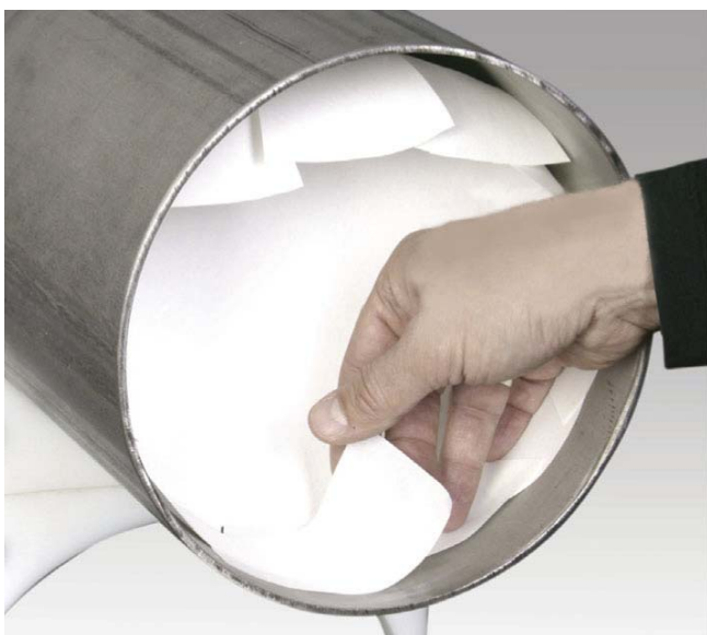
Figure 3. Insertion of handmade dam, made with Aquasol Water Soluble Paper.
