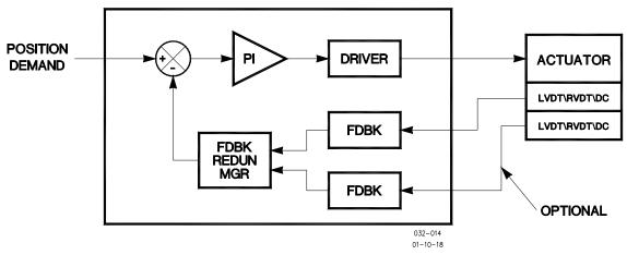
**Typical Integrating Actuator Block Diagram**
