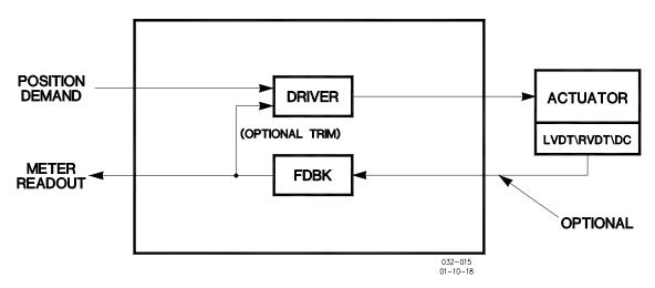
**Typical Proportional Actuator Block Diagram**
