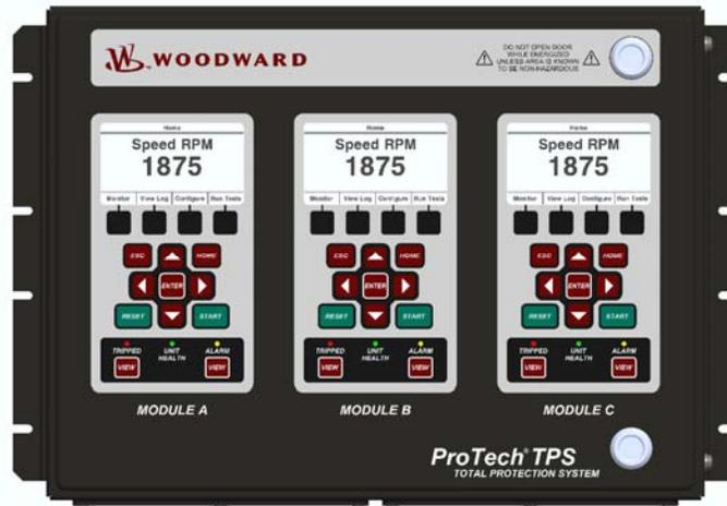
The ProTechTPS utilizes a triple modular redundant architecture and 2-out-of-3 voting logic to accurately determine unsafe conditions and ensure that no single-point failure will affect system reliability or availability. With this design, system failures (switches, transducers, modules) are detected, annunciated, and allowed to be repaired or replaced while the monitored system continues to operate on-line.
