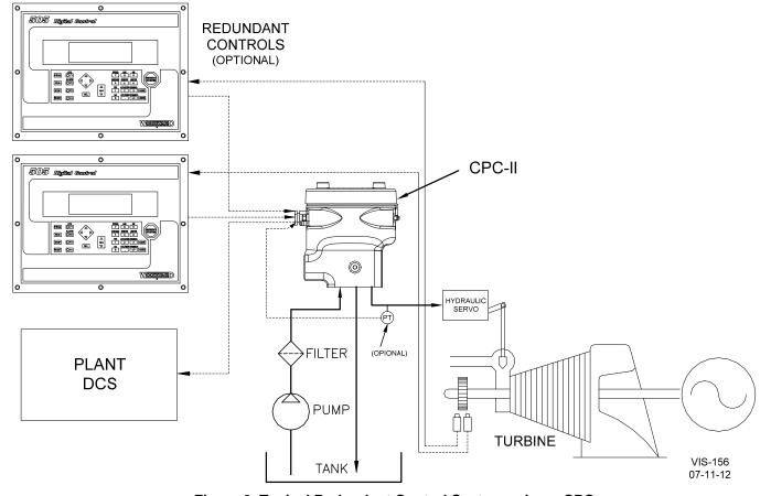
Figure 2. Typical Redundant Control System using a CPC
