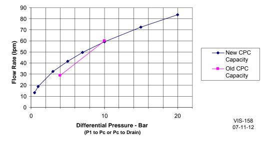
Figure 3. CPC-II Flow Capacity
