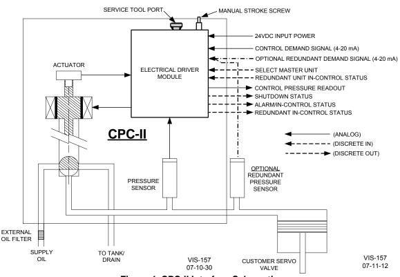
Figure 4. CPC-II Interface Schematic
