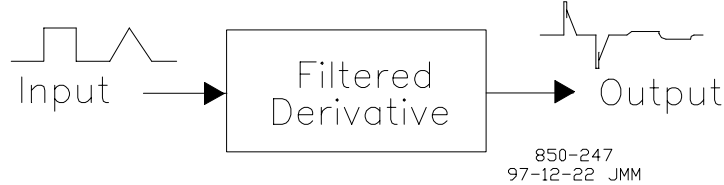
Figure D-5. The Derivative Term (Filtered)
