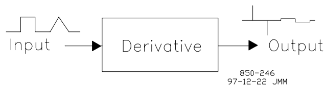
Figure D-4. The Derivative Term
