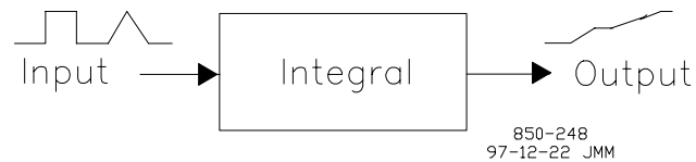
Figure D-8. The Integral Term
