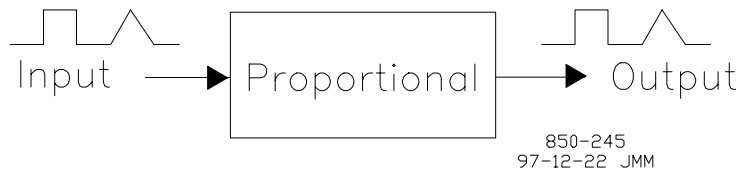
Figure D-1. The Proportional Term
