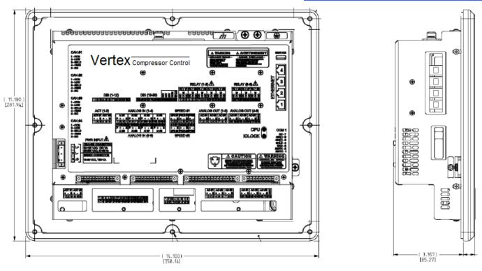
Figure 5. Vertex Control Package Dimensions
