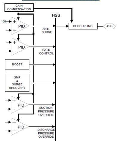
Figure 2. Basic Functional Control Diagram
