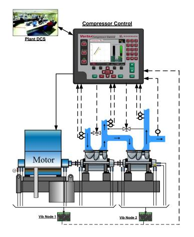
Figure 3. Typical Motor Driven Compressor Application (with two recycle loops configured)
