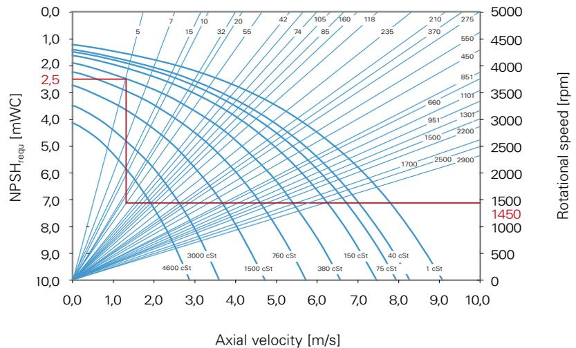
The NPSH-value (Net Positive Suction Head) indicates by how much the total pressure head at the pump inlet has to exceed the vapor pressure head  $p_d$  of the liquid to avoid cavitation. The available absolute pressure head is reduced by the suction head  $\Delta h_s$ , the pipe loss  $\Delta h_v$  and a safety margin of 2 mWC.
