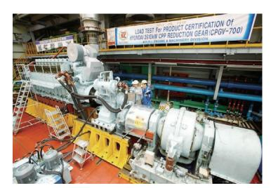
Loaded Gearbox Test with HiMSEN Engine (FPGV-660)
