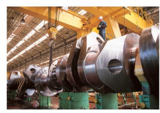
2-Stroke Diesel Engine Crankshaft Assembly
