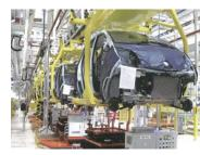
Engine Mounting RGV-Contactless
