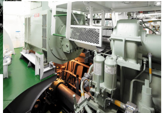
Using a generator driven by the speed reducer shaft.
