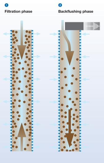
Flushing speed\* with candle open at both ends with throttle at top
