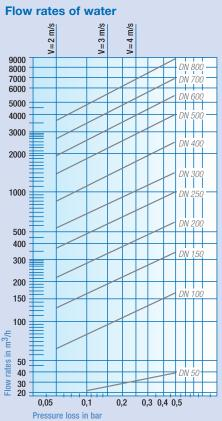
Of decisive importance for the design and sizing of a filter are the operational parameters. The size has to be selected on the basis of the flow rate, the degree of contamination, the filtration degree required and the permissible pressure loss in the filter. The diagram shows the flow rates with water at different nominal diameters at a filtration degree of 0.5 mm as a function of the pressure drop.
